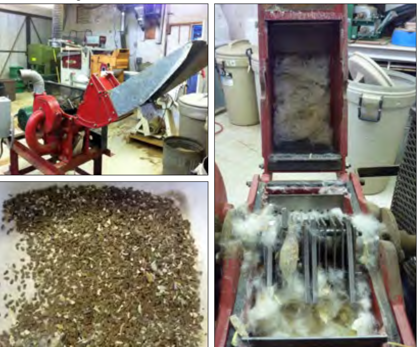
FIGURE 6.20: Hammermills can be used to process native thistle flowerheads similar to their use in processing other species such as milkweed (pictured here). Clockwise from upper left: Hammermill, partially processed milkweed ( Asclepias speciosa ) pods, milkweed seed lot condition after one pass through a hammermill.
