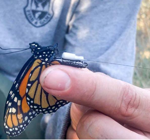
The Motus Wildlife Tracking System uses nanotags as light as 0.2 grams to track small birds and insects. The nanotag is a surveillance system that tracks the movement of the monarch, weighs about as little as a penny, and can transmit a signal to a tower that is about 15 miles away! **PHOTO:** IDFG
