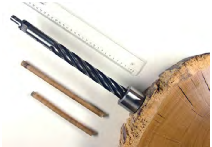
Drill for dendrochronology sampling and growth ring counting Creative Commons CC-BY-SA-2.5
