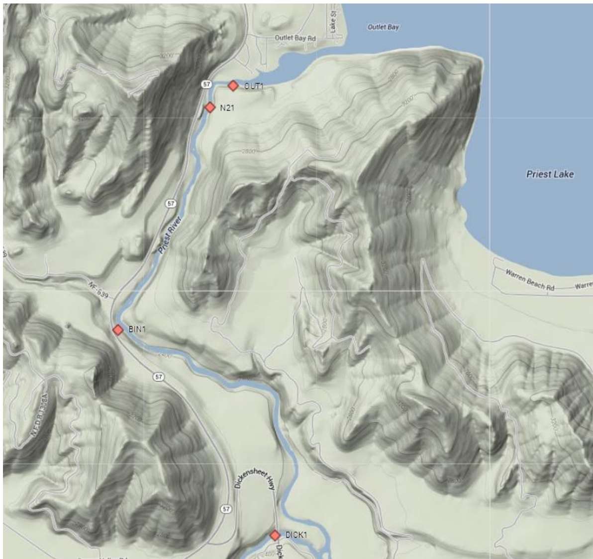
Figure 15: Priest River near the Priest Lake Outlet (OUT1). Flow rates at the upstream boundary at OUT1 were estimated by subtracting Binarch Creek flow rates (BIN1) from flow rate data or estimated flows measured at the Priest River near Cooling station (DICK1).
